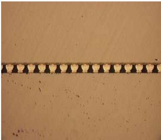
0.200mm Photo 2: 35 \mu m-pitch bumps mounting cross section
