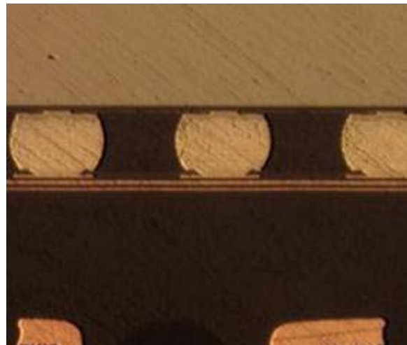
0.200mm Reference: 220 \mu m-pitch bumps mounting cross section
