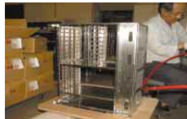
Use of stainless steel materials to replace coated parts at the Fujitsu Oyama Plant
