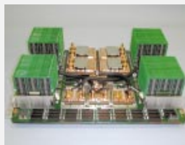
GS8900 Printed Circuit Assembly (Non-lead Solder is used)
