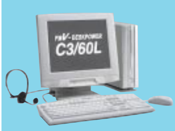
FMV-DESKPOWER C3/60L Recyclability ..... 93% Standby power consumption ..... 27W Uses recyclable paint All plastic parts of more than 25g marked
