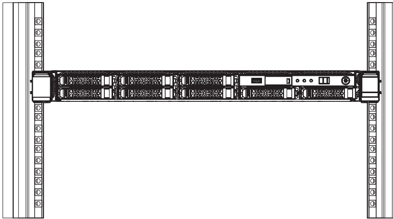
Figure 3-11 Completed SPARC M10-1 configuration
