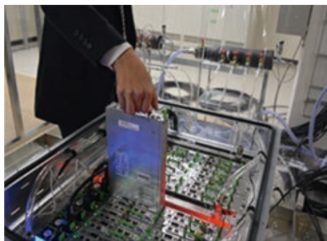
Liquid-immersion cooling technology to cool servers by submerging them in Fluorinert
