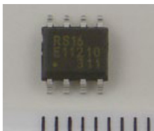
16K-bit Ferroelectric Lower capacity Random Access Memory (FRAM) product with Serial Peripheral Interface (SPI)
