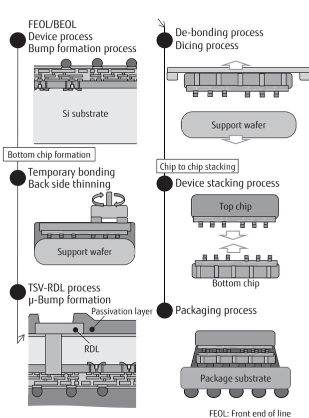
(a) Fabrication process flow of 3D LSI CPU module
