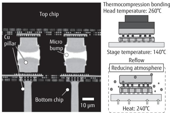
(a) Cross-sectional SEM image and process flow in micro bump stacking process
