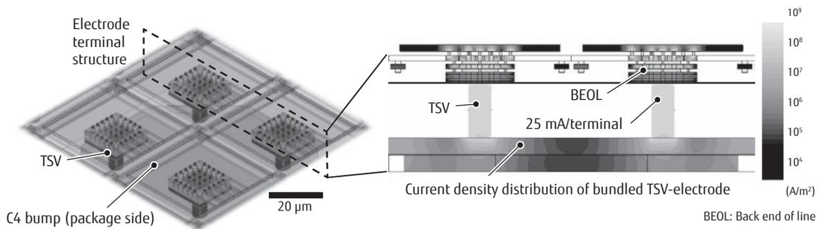
(a) Analyzing power cell current density of four-cell bundled electrode terminal structure
