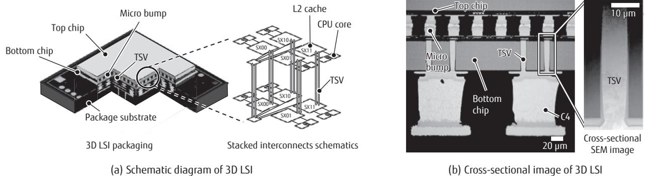
**Figure 1** Diagrammatic illustration and cross-sectional image of developed 3D CPU packaging module.
