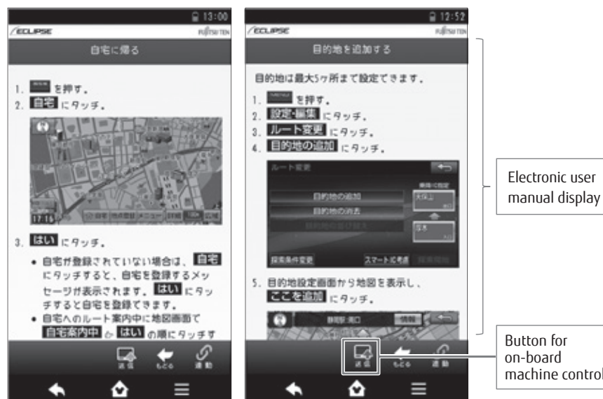
Electronic user manual display Function to control on-board machine Note) There is no English version of this app. As a reference, the Japanese version is shown here.
