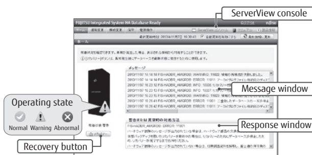
Figure 3 Display of operating state by Appliance Manager.
