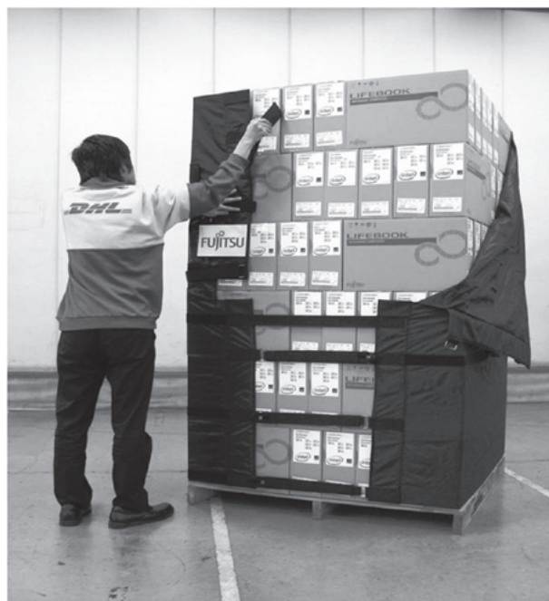
Figure 4 "Green Eco Belt" prevents stacked items from collapsing.
