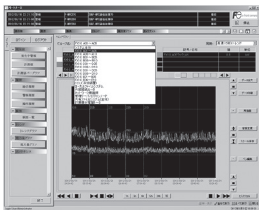
Figure 3 Power monitoring system screen.
