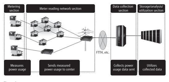
Figure 1 Overview of smart grid configuration.
