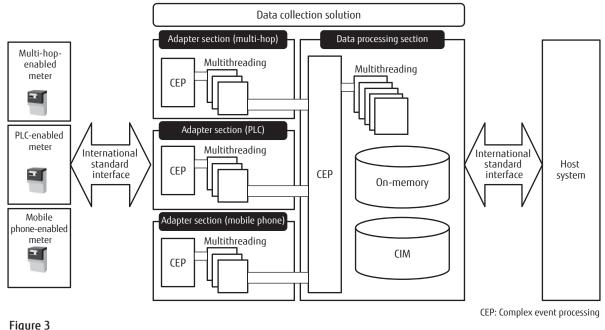
Data collection solution configuration and interfaces with devices and systems.
