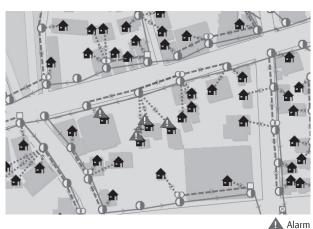
(b) Power failure monitoring/faulty facility identification screen
