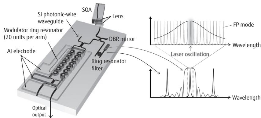
(a) Structure of integrated optical transmitter and laser wavelength selection mechanism
