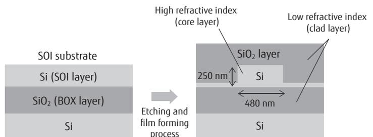
(c) Cross-sectional structure and manufacturing method of Si photonic-wire waveguide
