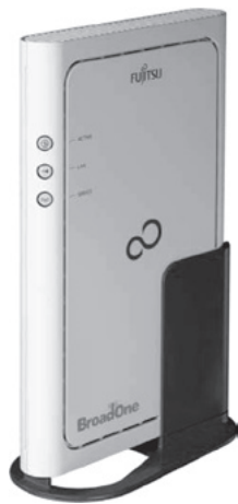
Figure 5 Appearance of femto base station equipment.
