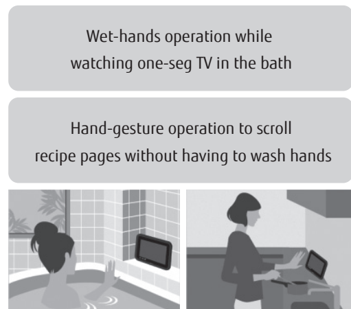
Figure 3 Device operation using hand gestures.
