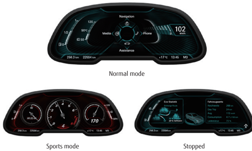
Figure 1 Instrument cluster using graphics.
