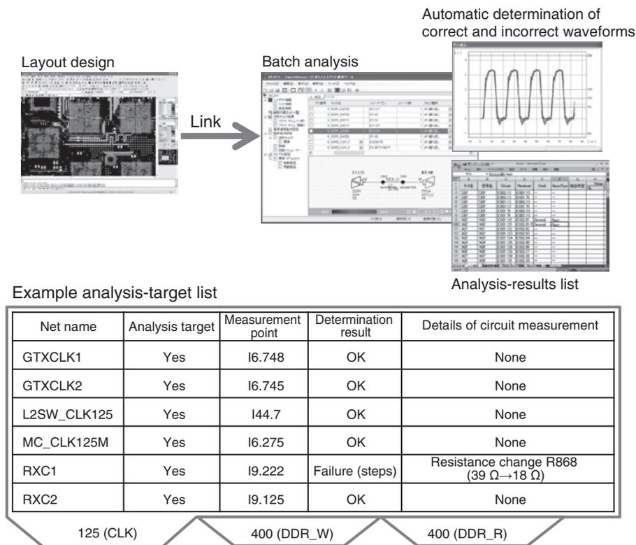
Figure 5 Example post-layout analysis.
