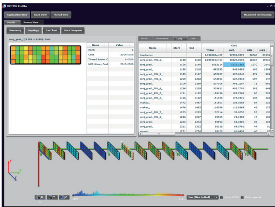
Figure 3 Screen shot 1 of cost analysis by basic profiler (topology display). Upper-left frame: cost information for each process (partial close-up) Upper-right frame: list of performance values for each program loop Bottom frame: cost information for each process (complete 3D topology display)
