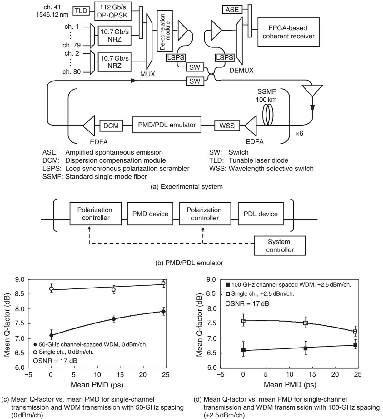
Figure 4 Experimental set-up for evaluating 112-Gb/s DP-QPSK signal and transmission characteristics.
