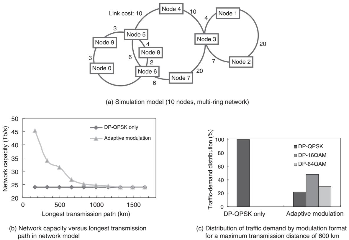
Figure 2 Characteristics of photonic network system using adaptive modulation technology.
