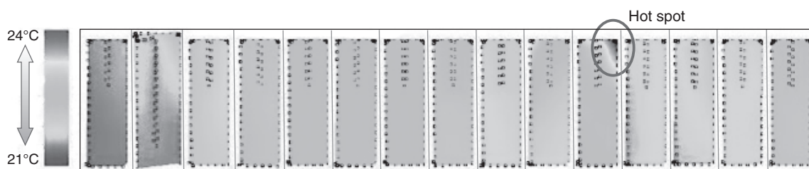
Figure 4 Example of measured temperature distribution on rack surfaces.
