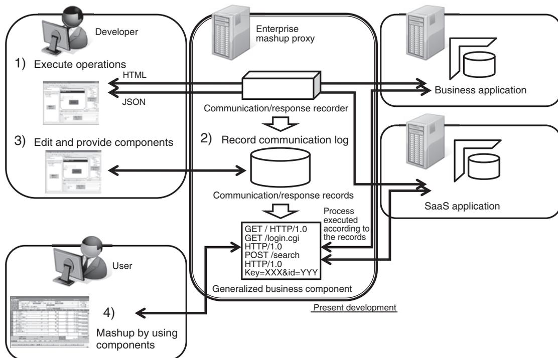
Figure 4 Overall support technology for making WebAPI.
