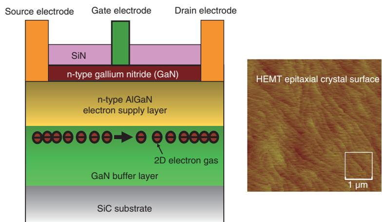
(b) Recessed-ohmic surface-charge-controlled GaN-HEMT structure
