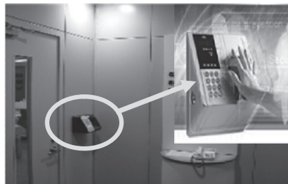
(b) Full security (access control by vein-pattern authentication)
