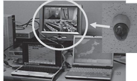
(d) Full security (entry recording by surveillance cameras)
