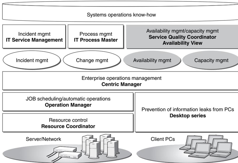
Figure 1 Systemwalker architecture.
