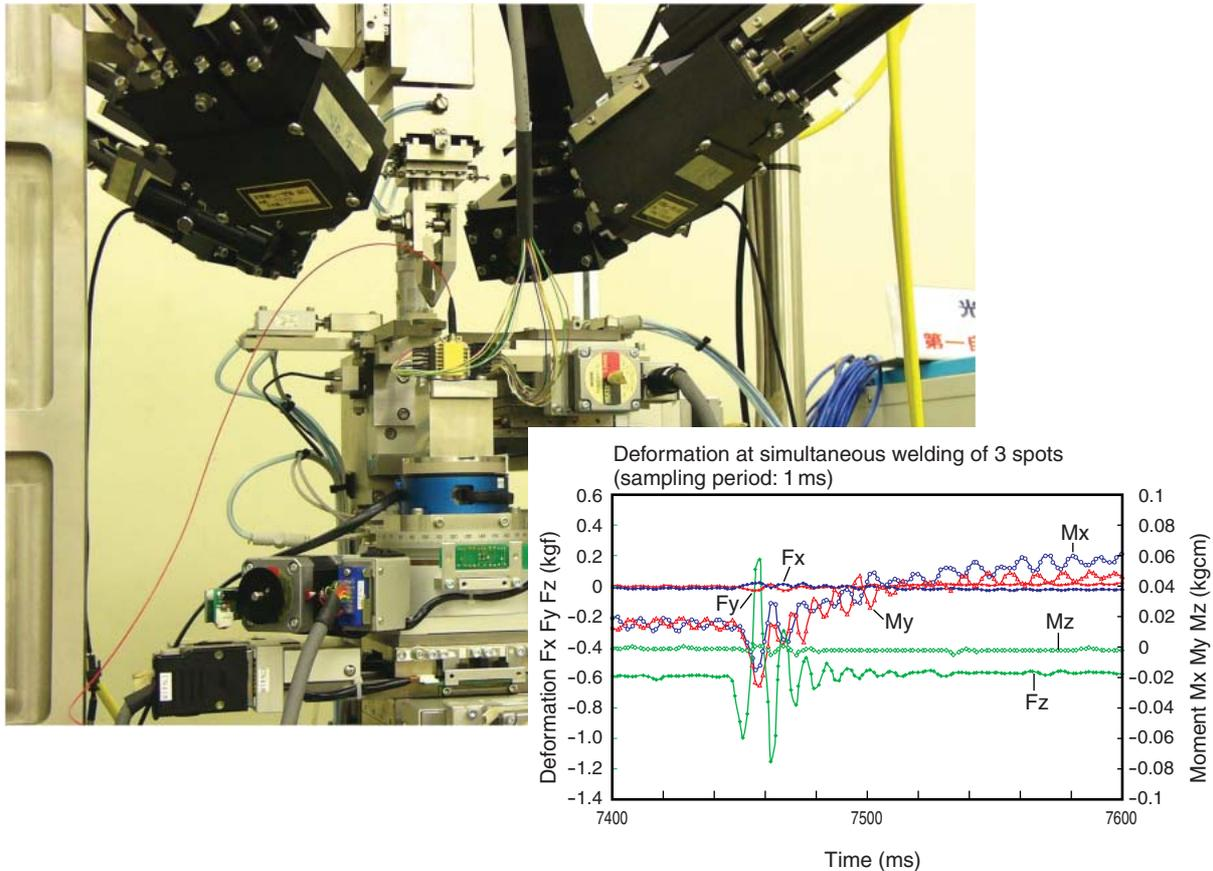
Figure 3 In-process monitoring of deformation at laser welding.
