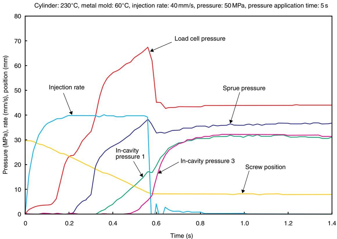
Figure 6 Monitoring of injection molding process.
