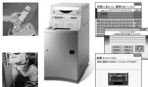
Figure 2 FACT-V automated teller machine.
