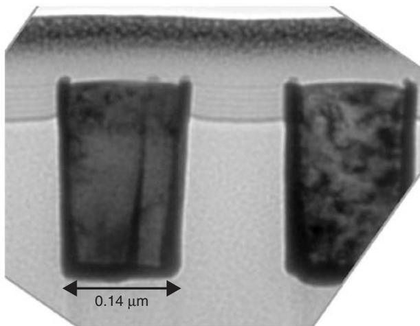
Figure 12 Cu electroplating structure without dishing and erosion.
