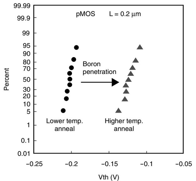
Figure 7 Threshold voltage distributions. At the higher temperature anneal, threshold voltage varies for the boron penetration.
