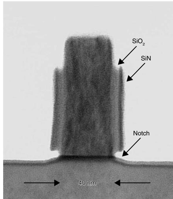
Figure 2 Cross-sectional TEM photograph of sidewall-notched transistor.
