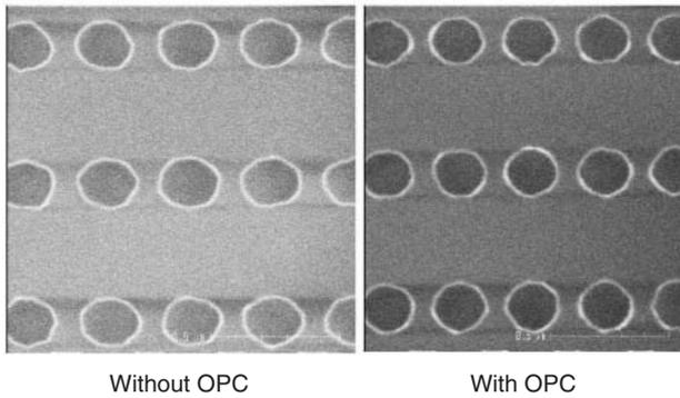
Figure 11 Effects of OPC in via patterning. Via shape is corrected from oval to circular by simulation-based OPC.
