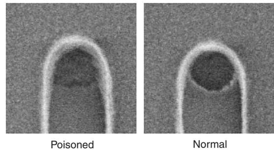
Figure 14 Line pattern resist at top of via.
