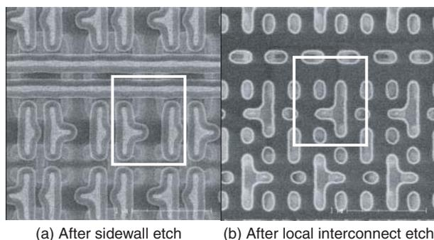
Figure 9 SEM photographs of high-density SRAM cell array. Cell size is  $0.9 \times 1.11 \mu\text{m}^2 (< 1 \mu\text{m}^2)$ .
