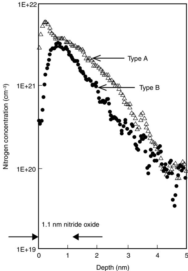
Figure 5 Nitrogen profile in nitrated oxide and substrate.
