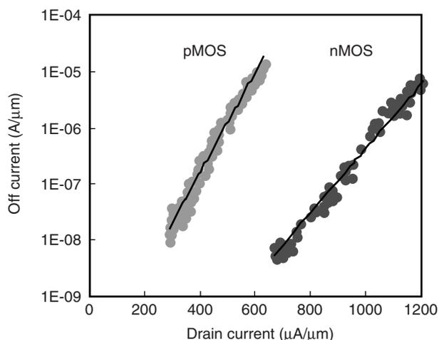
Figure 8 Ioff-Ion plots when supply voltage is 1.0 V.
