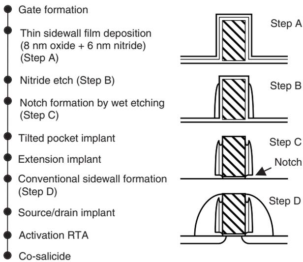
Figure 1 Sidewall-notched transistor fabrication.
