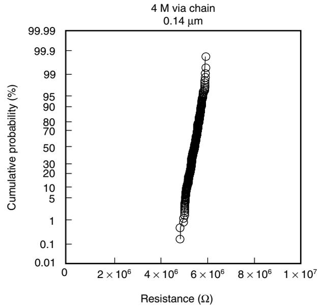
Figure 13 Via chain resistance of intermediate layer.
