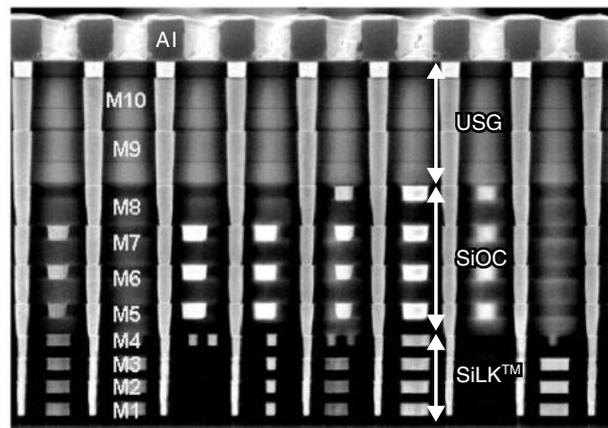
Figure 10 SEM image of 11 layers of interconnects.
