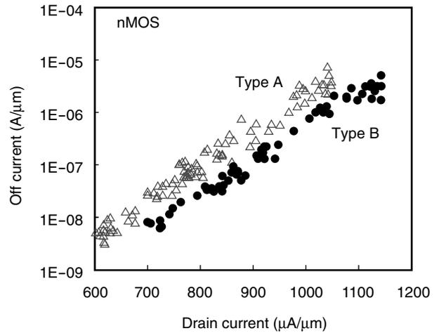
Figure 6 I<sub>off</sub>-I<sub>on</sub> plots for nMOS when supply voltage is 1.0 V. See Figure 5 for Type A and B.
