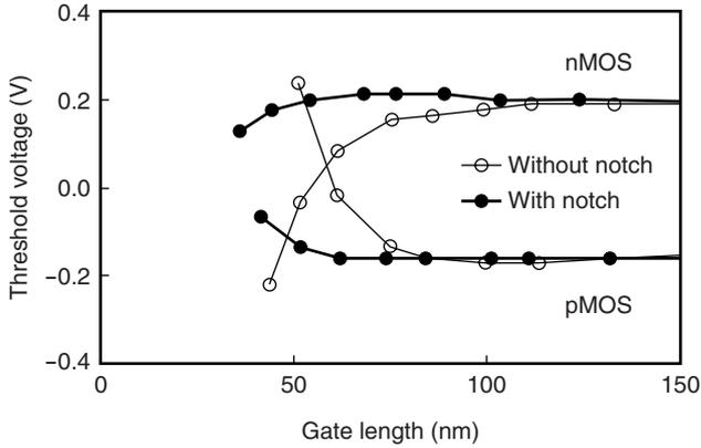
Figure 4 Improved roll-off characteristics of transistors with sidewall-notched gate electrode.
