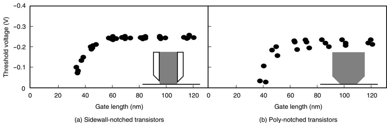
Figure 3 Threshold voltage as a function of gate length (pMOS). Sidewall-notched gate structure suppresses variations of threshold voltage.
