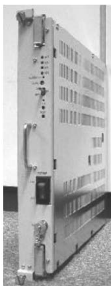
Figure 9 High-efficiency TX-AMP (with digital predistorter).
