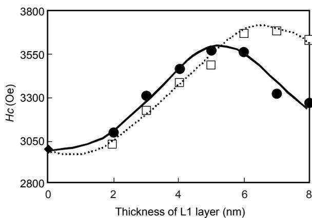
Figure 6 Dependence of coercivity on L1 layer thickness for SFM structures [L2/Ru/A] (open squares) and [L2/Ru/B] (solid circles).
