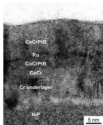
Figure 2 Cross-section TEM image of an SFM with two CoCrPtB layers separated by 0.8 nm of Ru (dark band).
