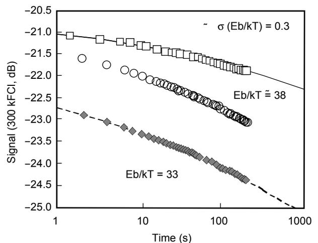
Figure 4 Signal decay at room temperature for 300 kFCI bits in various SFM: [12/Ru/4] (open squares), [12/Ru/4] (open circles), and 12 nm-thick single layer (solid diamonds). Lines are fitted to a model.
