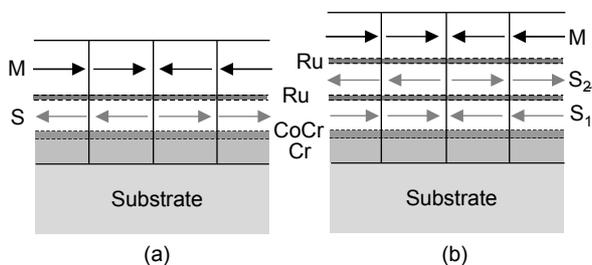
Figure 1 Schematics of the SFM structure with (a) one ( $S = L1$ ) and (b) two ( $S_1$  and  $S_2$ ) stabilizing layers disposed between the main magnetic layer ( $M = L2$ ) and the CoCr and Cr seed layers. Interlayer antiferromagnetic coupling is mediated by the thin Ru layers.
