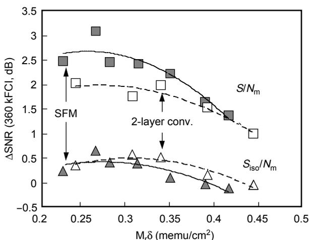
Figure 8 Medium SNR of two-layer SFM (solid symbols) compared with two magnetic layer conventional media (open symbols). The values given are relative to a medium on NiP/Al-Mg used for a 20 GB/platter drive.
