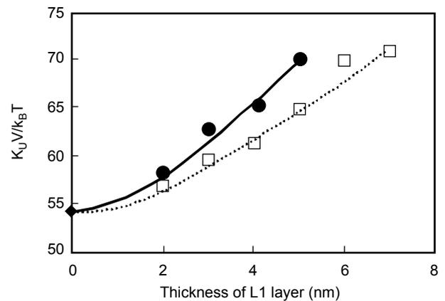
Figure 7 Plot of stabilization factor  $K_u V/k_B T$  vs. thickness of L1 layer for SFM structures [L2/Ru/A] (open squares) and [L2/Ru/B] (solid circles).
