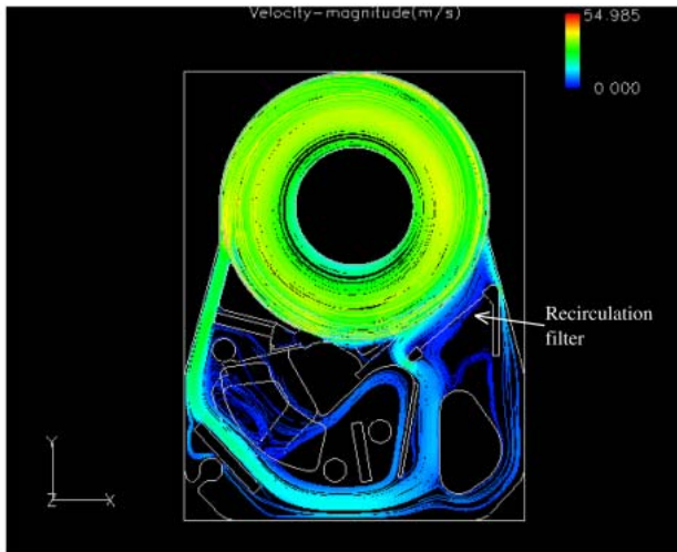
Figure 17 Streamline plot in AL-7LX (15 krpm).
