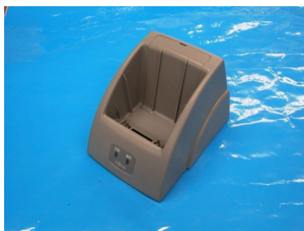
(a) Communication interface unit
