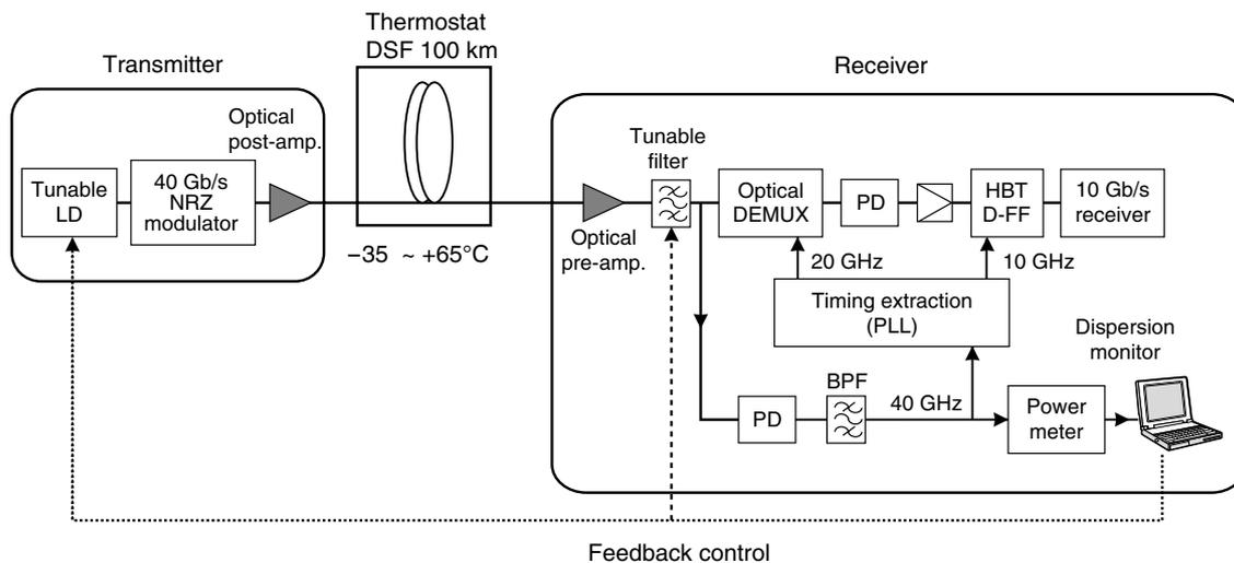
(a) Setup of automatic compensation experiment
