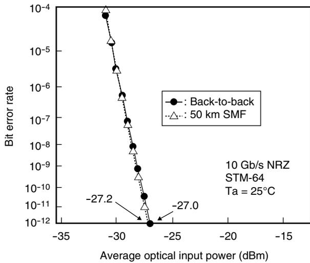
(b) SMF 50 km transmission with no sensitivity degradation
