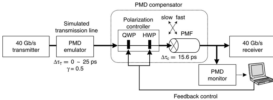
(a) Setup of automatic PMD compensation experiment
