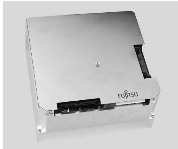
Figure 5 Photograph of proposed WDM amplifier.
