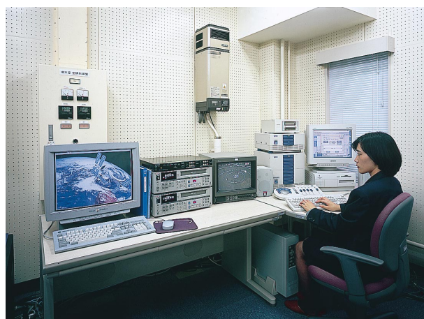
Fig.3— Image processing workstation Power ONYX (SGI), and video editing system Turbo CUBE
