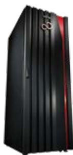
FUJITSU Storage ETERNUS DX8000 S3 series disk storage system
