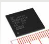
MB86E631 interface bridge SoC with 10 different built-in interfaces
