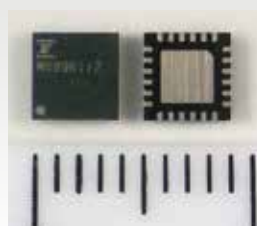
MB89R112 HF-band RFID tag with built-in FRAM
