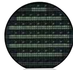
6-inch silicon wafer used to form GaN power device
