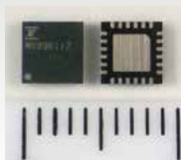
MB89R112 HF-band RFID tag with built-in FRAM
