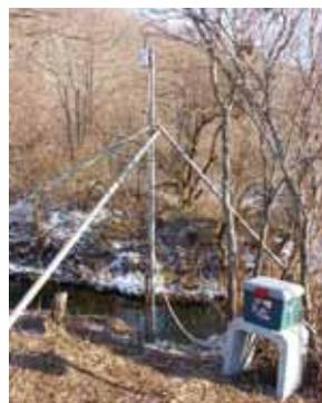
Multi-sensing unit installed at natural feeding ground for Japanese cranes
