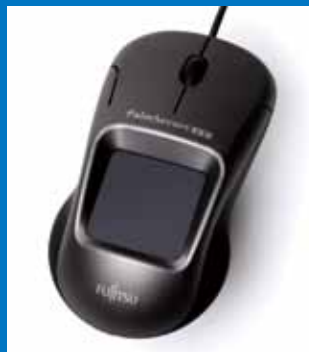
PalmSecure-LT palm vein biometric authentication device (mouse sensor-type) exclusively for PC login
