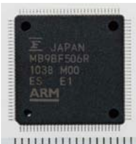
The FM3 family of 32-bit general-purpose RISC microcontrollers use ARM's Cortex™-M3 core
