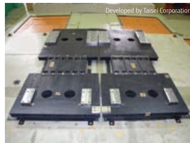
Vertical furnace installed with a seismic isolation platform
