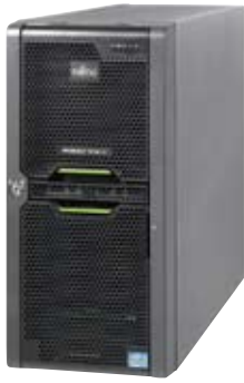
PRIMERGY TX140 S1 1-way tower x86 server
