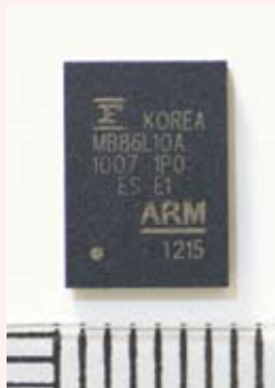
RF transceiver LSI for mobile phones compatible with LTE, a next-generation communications format
