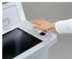
Palm vein authentication in use at an ATM
