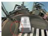
Sample view when turning left: perspective from above-rear (clearly shows curb clearance of left rear)
