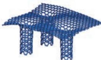
Structure of new nanocarbon composites
