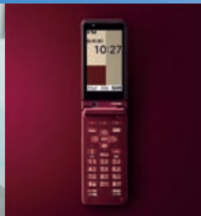
The Raku Raku Premium mobile phone enables users to dictate email by voice
