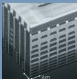
Advanced, multilayer wiring used in LSI devices
