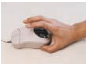
Biometric mouse with palm vein pattern recognition device
