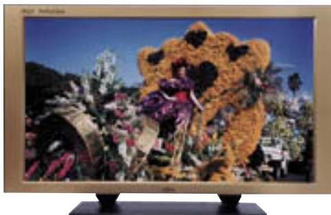
42-inch PDP with ALiS technology for HDTV use
